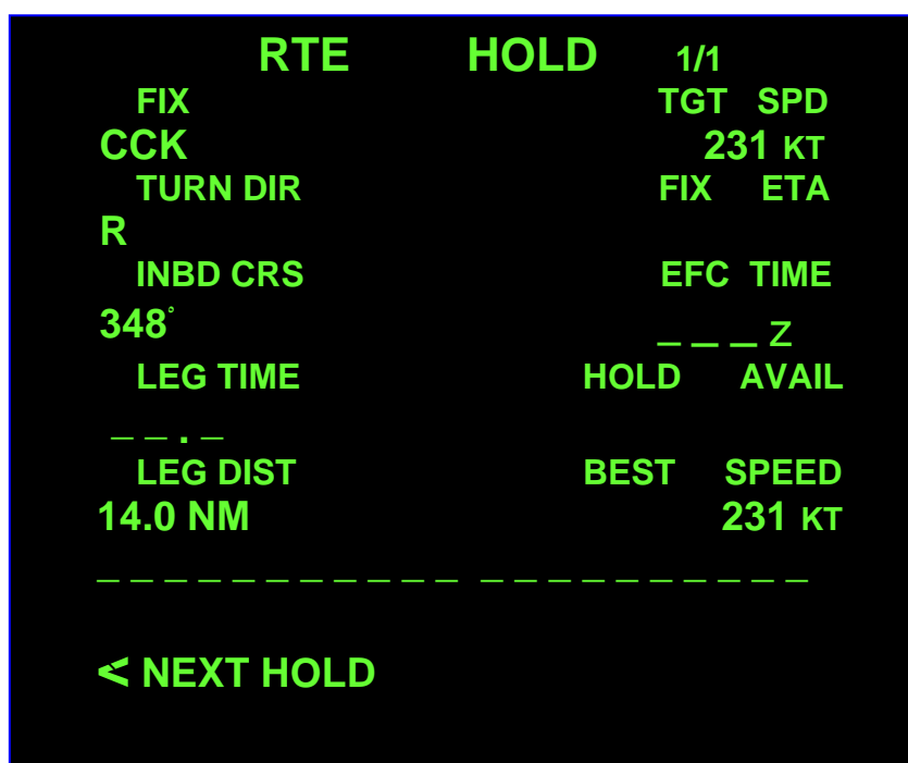
Figure 6: FMC CDU display showing hold page after leg distance had been entered.
