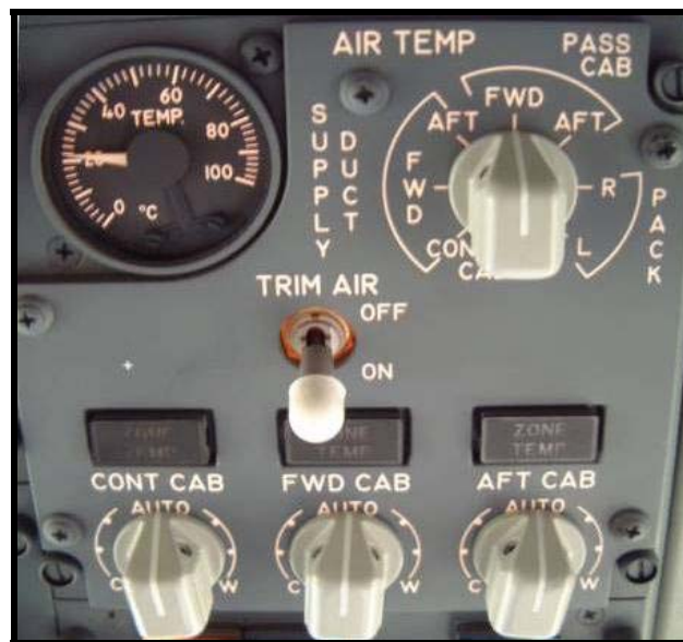
Figure 1: Boeing 737-800 series aircraft air conditioning control panel showing the three zone temperature selectors and supply duct temperature gauge. 21
