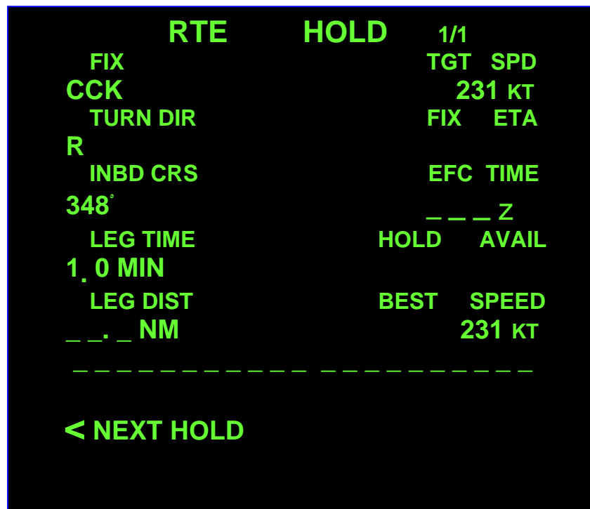
Figure 5: FMC CDU display showing hold page before leg distance had been entered.
