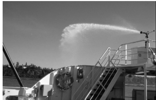
Figure 7 - Kuper Fire Monitor Installation – water stream directed overboard
