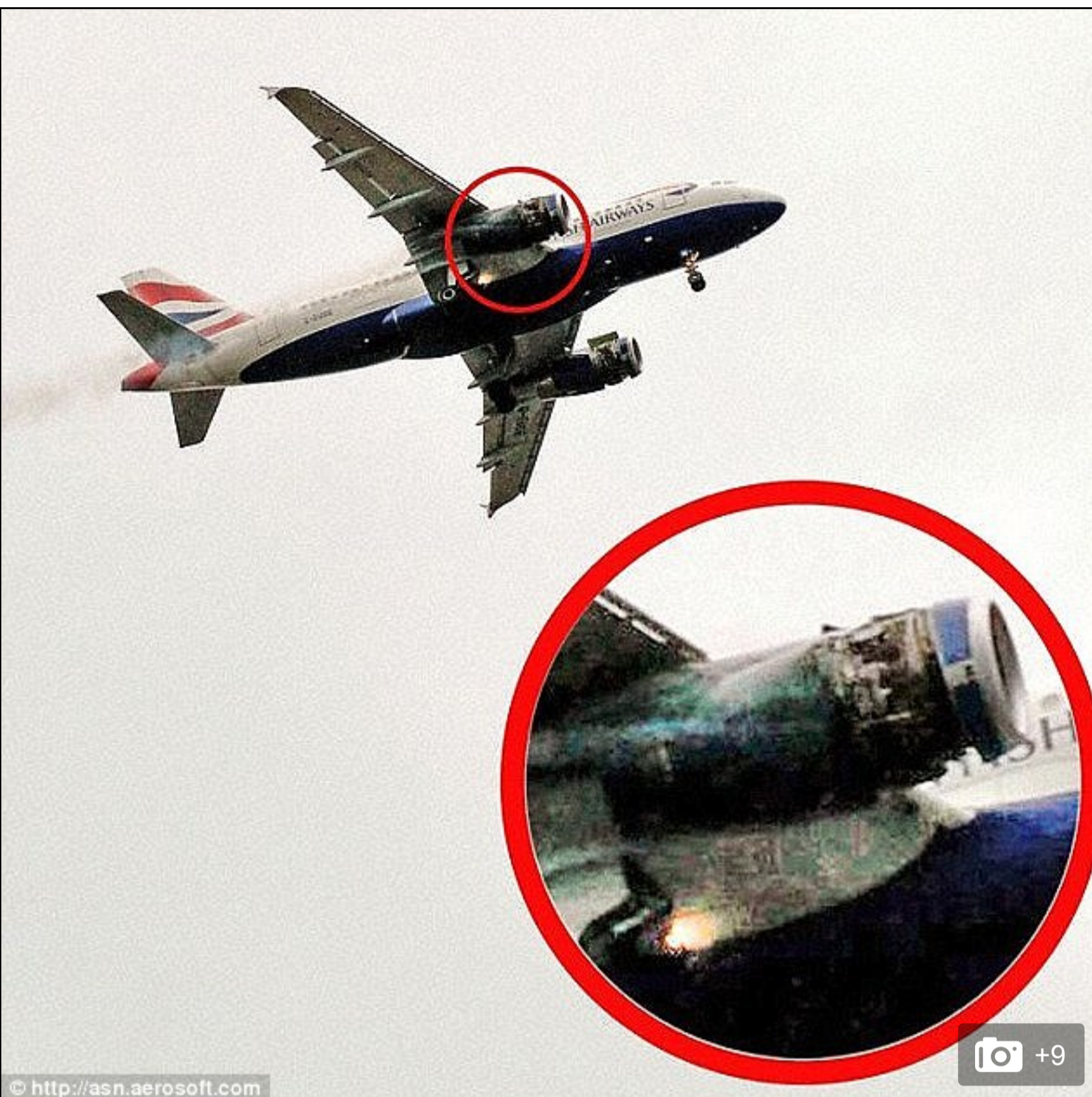
On fire: Passengers were left terrified when the covers of both engines blew off and one of them burst into flames on the flight of an A319 from London to Oslo in May 2013
