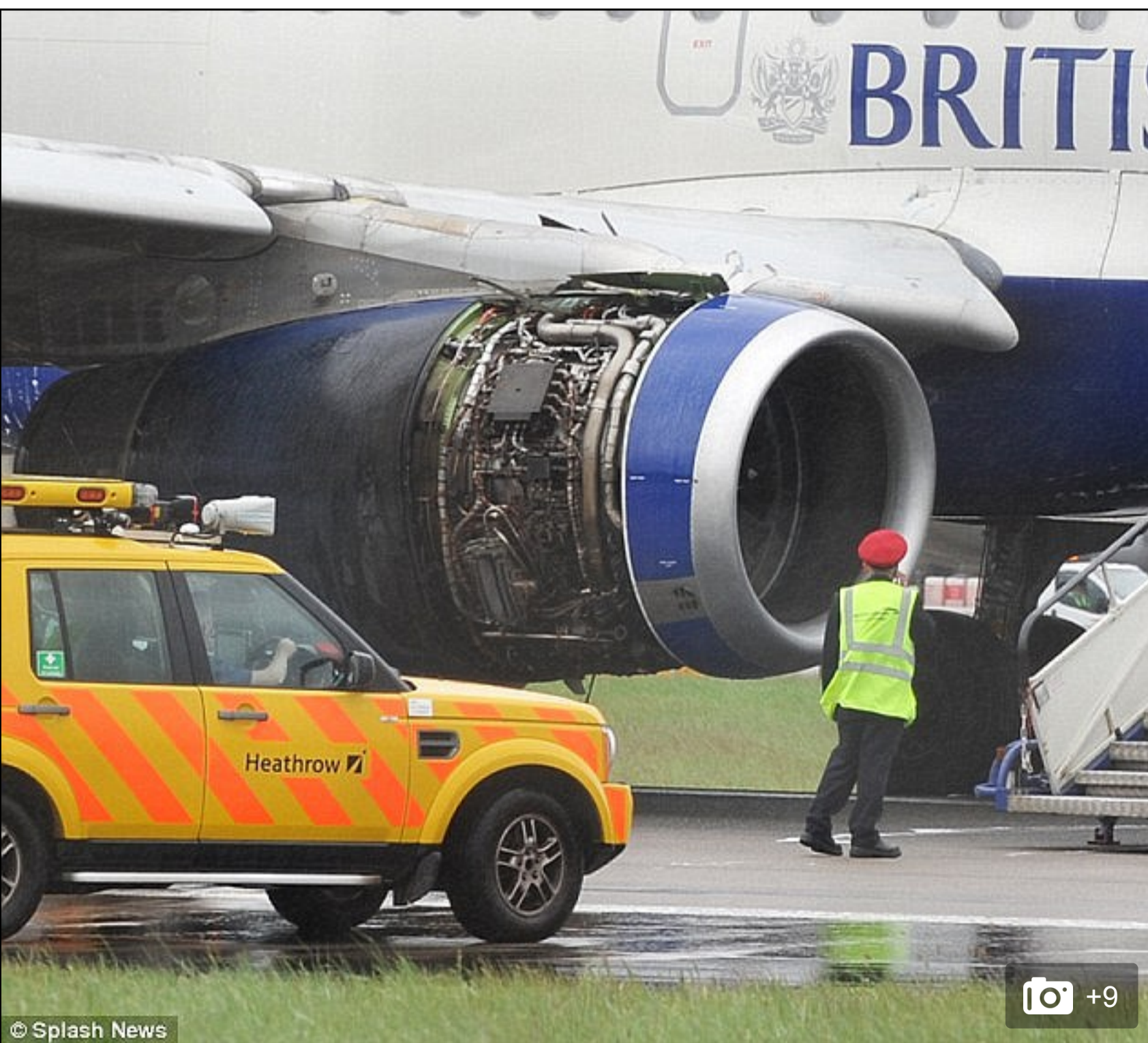
Engineers 'failed to lock doors on both engines' which resulted in the emergency landing
