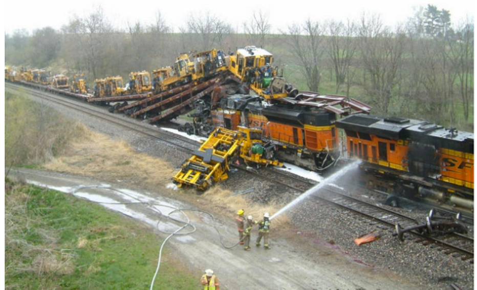
Firefighters spray the wreckage of a 2011 collision between a BNSF coal train and an equipment train. The collision was caused by crew fatigue. Photo courtesy of NTSB/Red Oak Fire Department
