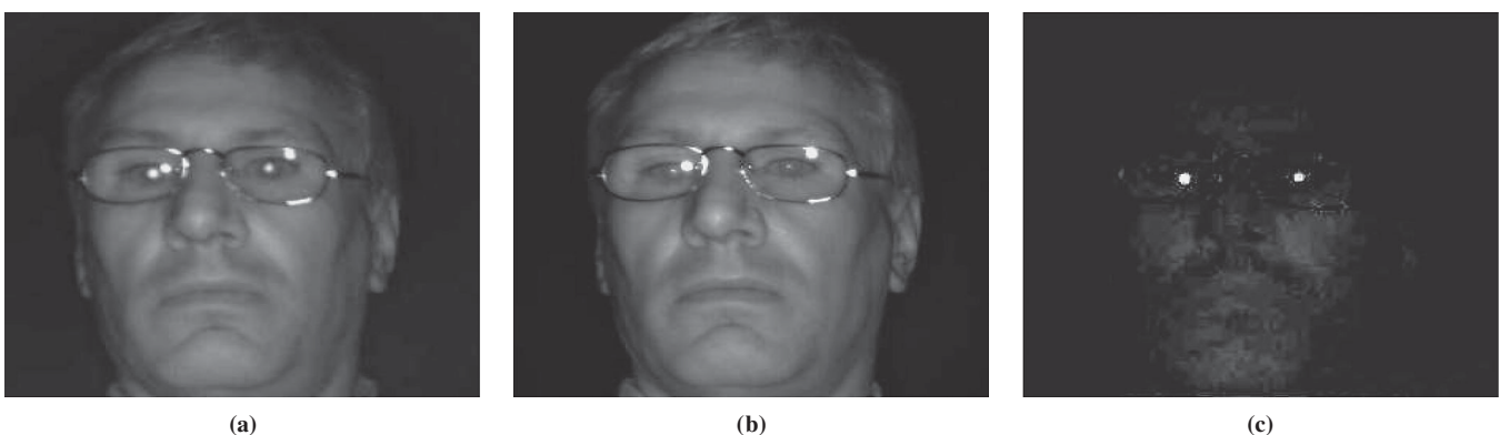
FIGURE 2 Eye images taken by CoPilot: (a) bright-eye, (b) dark-eye, and (c) difference images.
