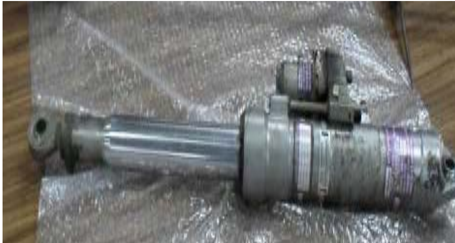
Photo 17: Leading Edge Flap Actuator
