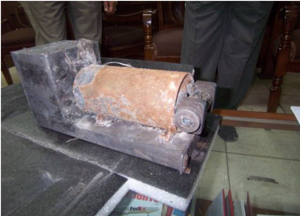
Photo 6: Damaged CVR Recovered From the Crash Site
