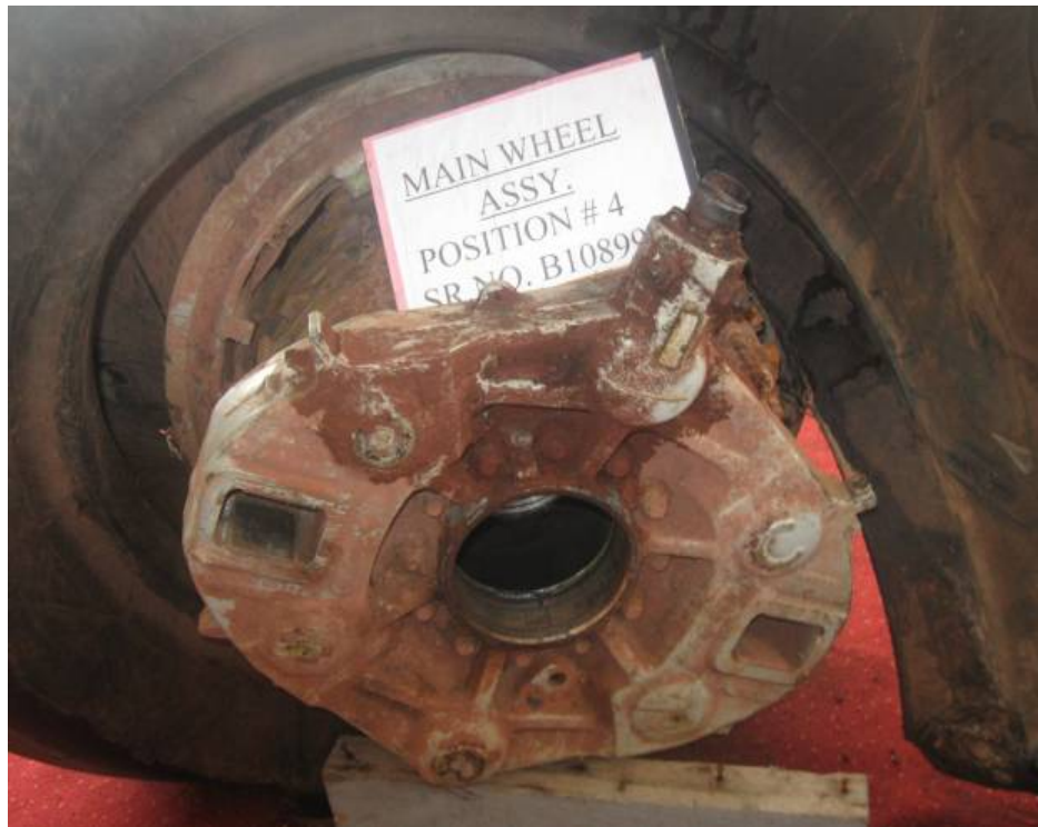
Photo 28: Main Wheel and Tyre Assembly
