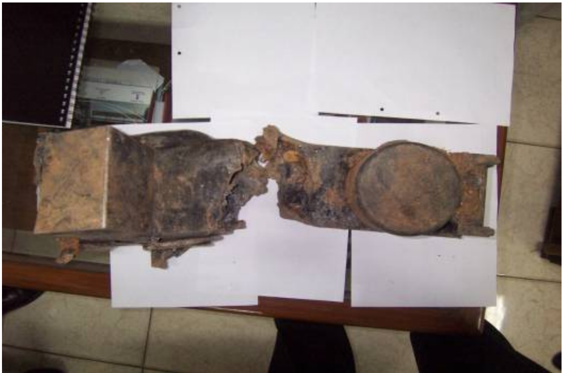
Photo 4: Digital Flight Data Recorder (In Damaged Condition)
