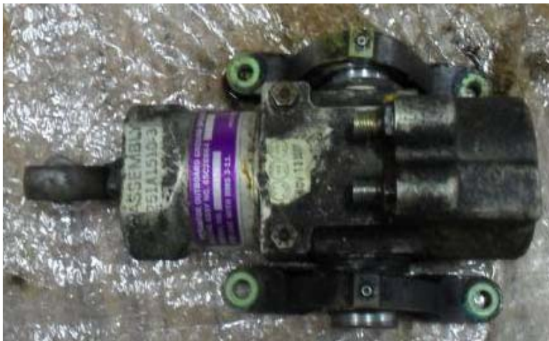
Photo 19: Ground Spoiler Actuator
