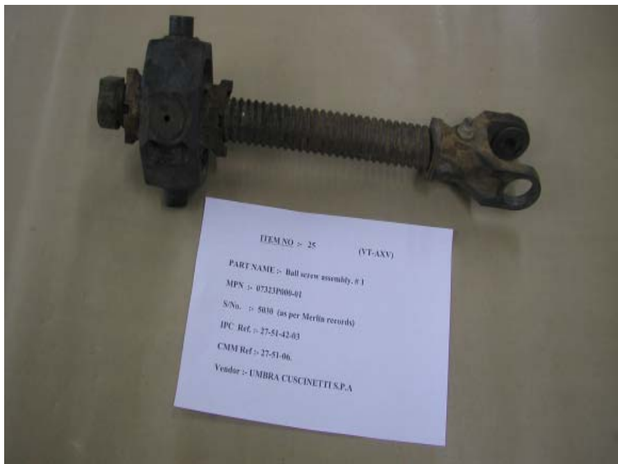
Photo 20: Trailing Edge Flap Ball Screw
