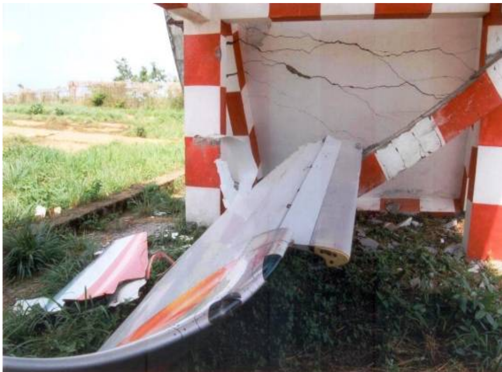
Photo 10: Broken Wing of Aircraft after Impacting the ILS Mounting Structure
