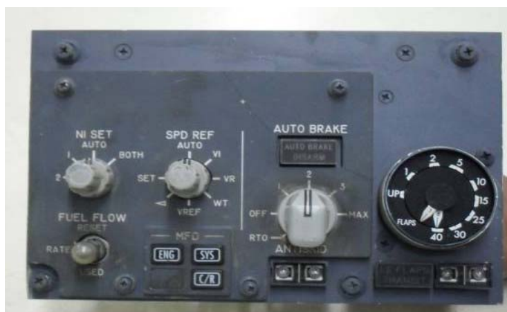
Photo 16: Brake Selector Panel and Flap Position Indicator
