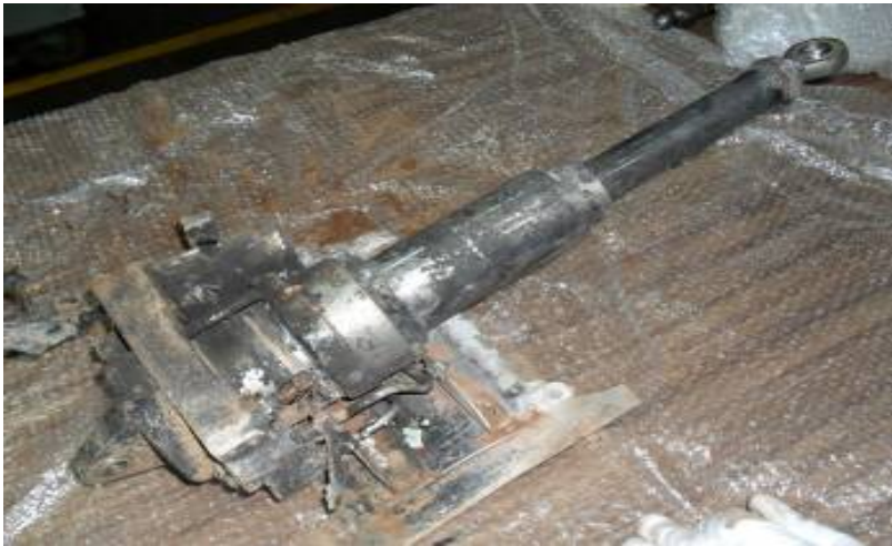
Photo 18: Leading Edge Actuator Assembly
