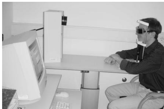
Fig. 1. Experimental setup for the pupillography. The patient wears an infrared protective goggle, has propped his chin on a device and looks toward the infrared camera.
