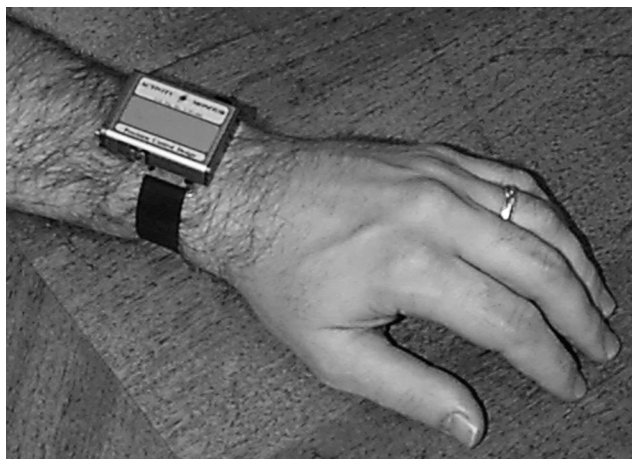
Fig. 3-3. One type of wrist-worn actigraph for the measurement of movement during field operations. From the measurement of activity, it is possible to make predictions of sleep obtained by soldiers using automated sleep-scoring algorithms.
